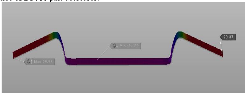
Figure 3: The effect of the blank holder force 30 kN on the springback.
